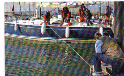
8 RIGHT: Motoring on the beam spring brought the boat even closer to the windward side and increased our safety margin away from the downwind dangers
