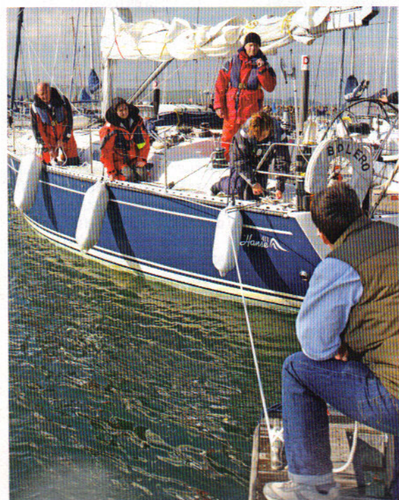
7 BELOW: About three metres from the windward side, the line was made fast. Whilst the boat hung stern to wind, excess lines and fenders were tidied, and we re-briefed for the next crucial stage. The temporary rope fairlead was released to make the stern line become a beam spring. The stern drifted downwind and the boat swung beam to wind
