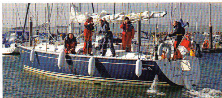
9 ABOVE: When positioned to windward, the beam line was released ashore – retrieved on board – and the engine powered up once again to gain steerage way. Heart rates began to fall once we'd gained momentum. With lines and fenders stowed, we headed for the lumpy stuff with a scrap of jib. Fifteen minutes later the engine was on again, as the wind had died completely!
