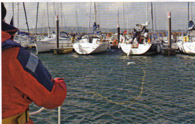
3 ABOVE: To pre-rig the line we'd use to turn the boat, a crew member floated the throwing line connected to a warp and fender across the marina aisle to the boat
