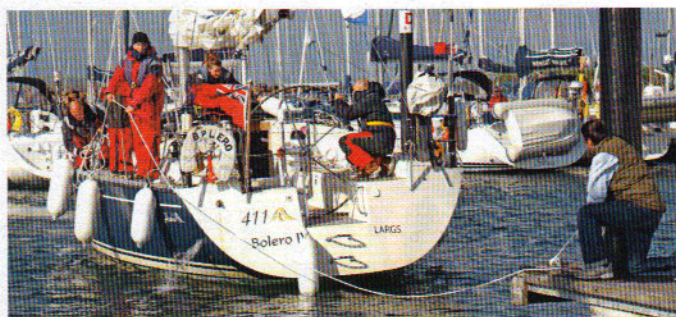
5 ABOVE: We released our stern line and bow spring and reversed out. As the boat moved astern, slack in the line was taken up onboard to keep it clear of the prop and rudder
